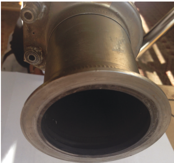
Bleed air off take port from a Boeing 737. Interior is black from oil contamination.
