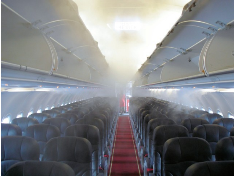
Condensation on AirAsia flight AK6303 with A320 from Langkawi (LGK) to Kuala Lumpur (KUL). Departure in tropical rainforest climate ("PlaneHunter", http://bit.ly/2oUJYKP )
