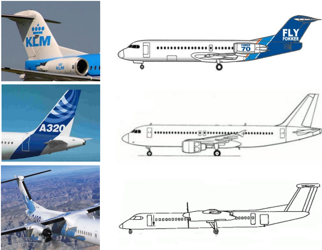
Fig. 12 – Examples of dorsal fin geometries. From top to bottom: (a) standard dorsal fin, (b) round edge dorsal fin, (c) dorsal fin with dorsal fin extension. Aircraft: (a) Fokker 70 [19-20], (b) Airbus A320 [21-22], (c) Bombardier Q400 [23-24]
