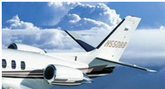
Figure 2.23 3D view and side view of a dorsal fin with air intake ram of a Cessna Citation Bravo ( Stajets 2013 and Aviastar 2013b )
