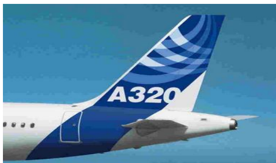
Figure 2.22 Side views of a round edge dorsal fin of an A 320 ( Prendrel 2013 and Aerospaceweb 2013 )
