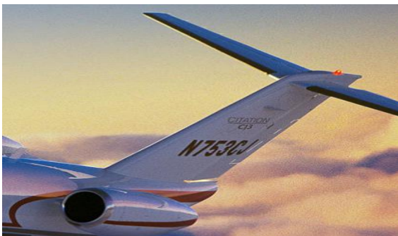
Figure 2.20 3D view and side view of a conventional tail (with a sharp leading edge) of a Cessna Citation CJ3 ( Automobile 2013 and Blueprints 2013 )
