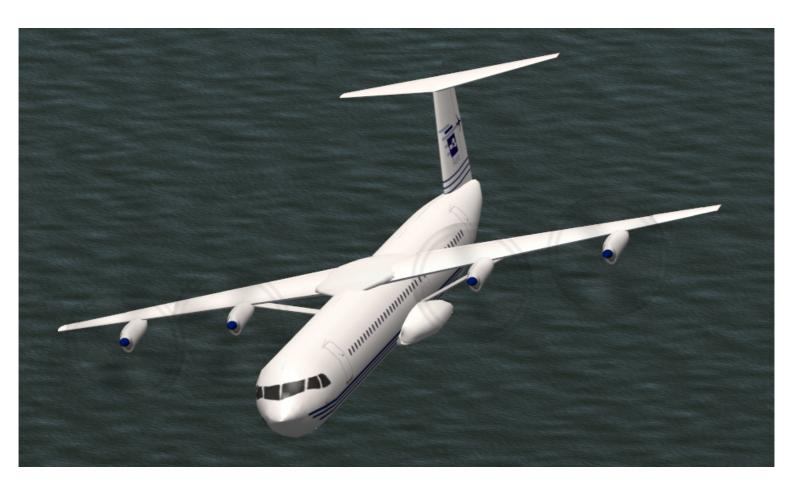
"Smart Turboprop" with Wing Brace (4 Engines)
