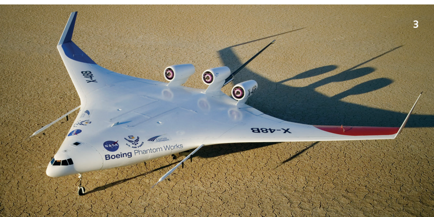
3 Boeing X-48B unmanned blended wing body demonstrator [3]
