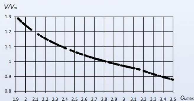
Fig. 6 Speed-to-minimum drag speed ratio, V/V_m as a function of maximum lift coefficient for landing configuration, C_{LmaxL} .
