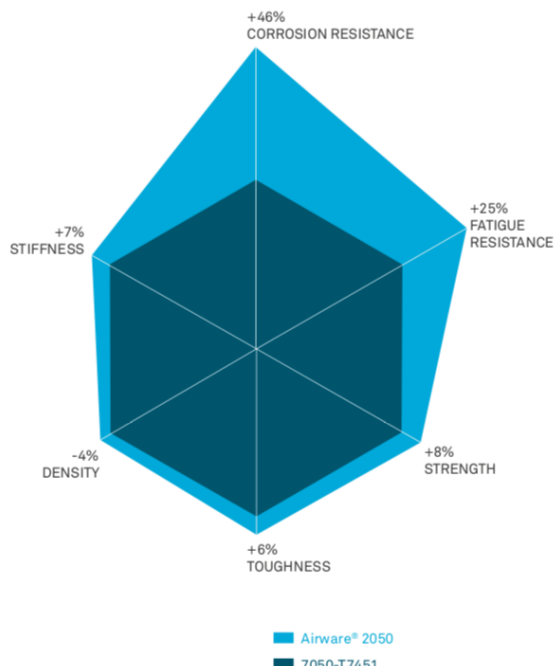
Figure 12.4 Comparison of the properties of Airware 2050 with a conventional aluminium-copper plate of 75mm thickness (Constellium 2017)
