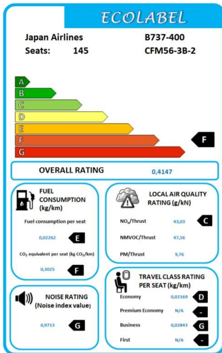
Figure 6.17 Example of one ecolabel calculated by Van Endert. Extracted from (Van Endert, 2017)
