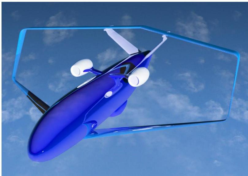
Figure 4.2 Box wing aircraft concept (Aero 2013)
