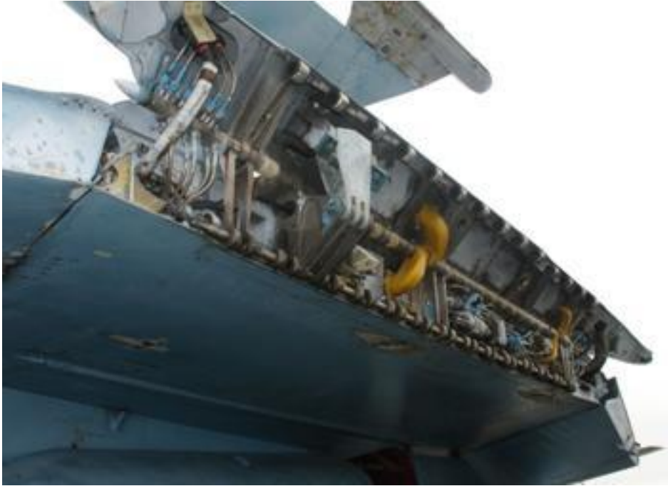
Figure 3.19 Folding system installed on a wing (Yarygina 2013)
