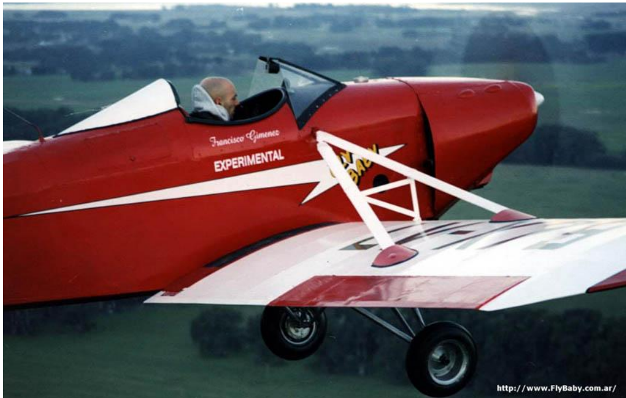
Figure 2.4 Modified Fly Baby with top struts (FlyBaby 2013)
