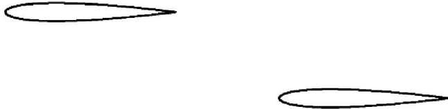
Figure 2.4 Positive stagger of a biplane
