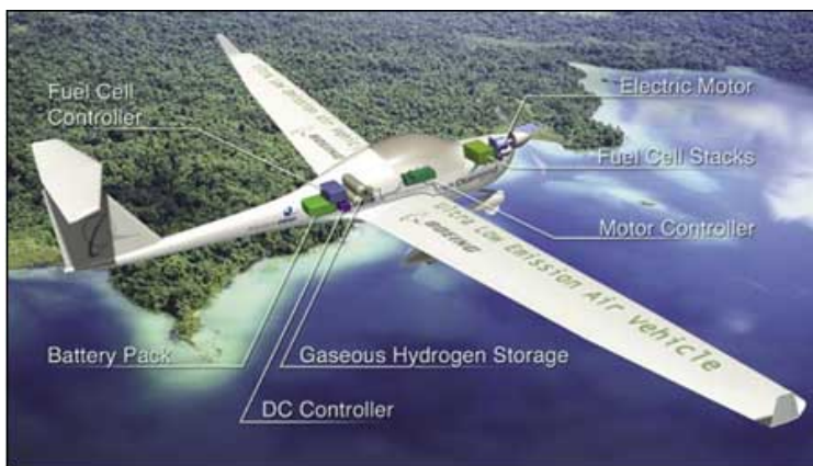
Figure 2.10 Principal Drawing of Boeing's Fuel Cell Demonstrator airplane ( Boeing 2003 )
