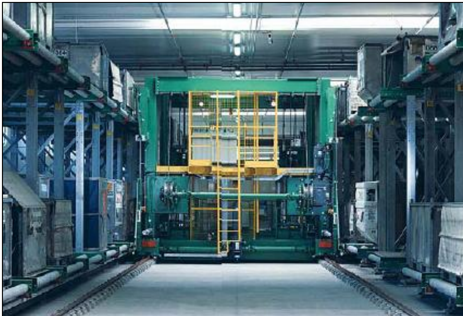
Figure 2.13 Freight storage by elevating transfer vehicles (Siemens 2006)
