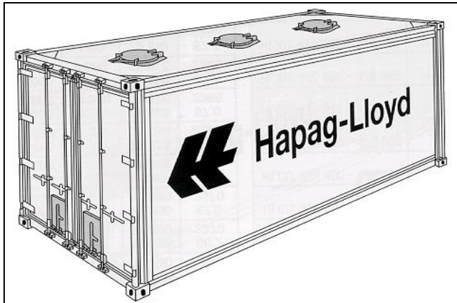
Figure 3.19 20-ft bulk container with three loading hatches in the roof (GDV 2007)
