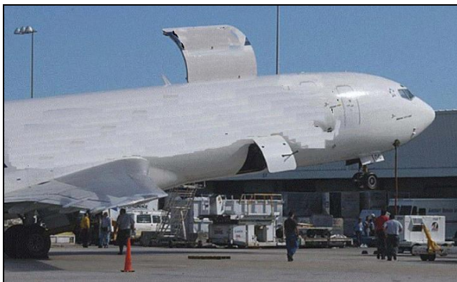
Figure 2.19 Improper loading (Young 2007)
