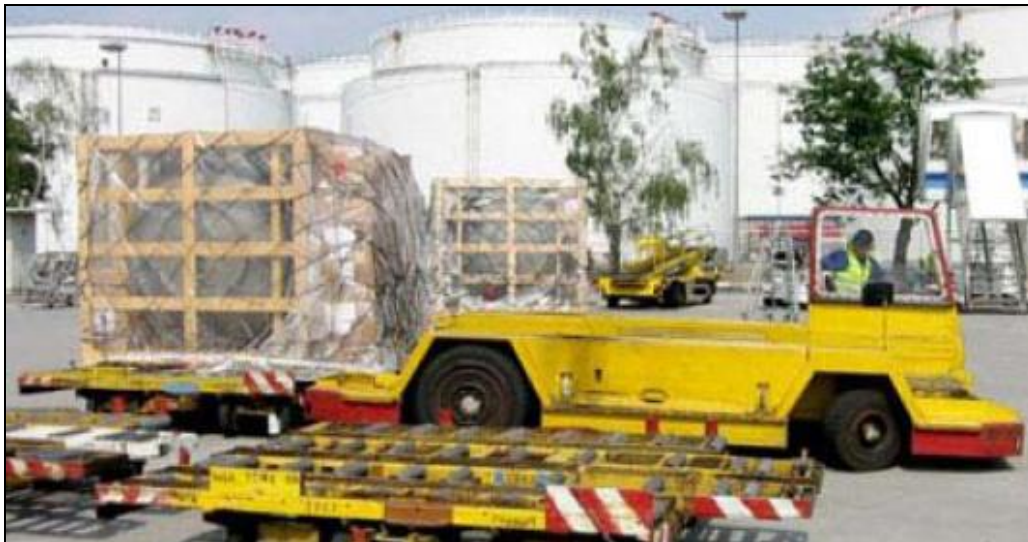
Figure 2.17 Transfer of a pallet from a dolly to a transporter ( GDV 2006 )
