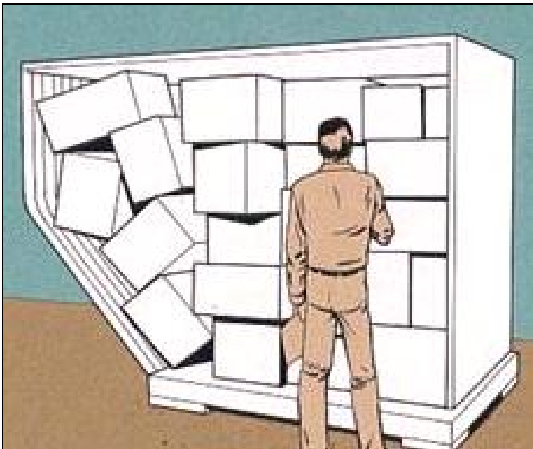
Figure 3.3 Stacking problem of containers ( Inamar 2007 )
