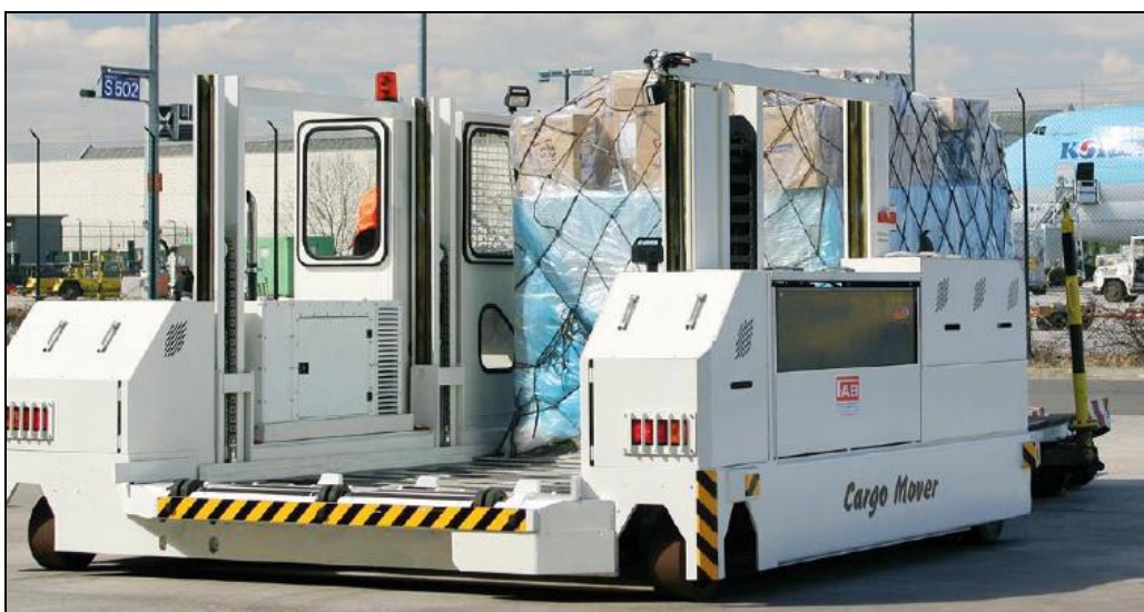
Figure 2.18 The multifunctional FAB – cargo Mover ( FAB 2007 )
