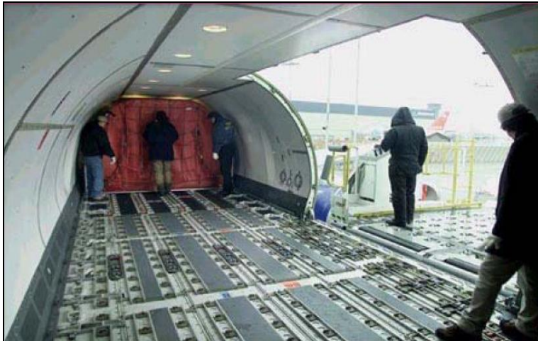
Figure 2.15 B757: Side door loading ( Haggerty 2004 )
