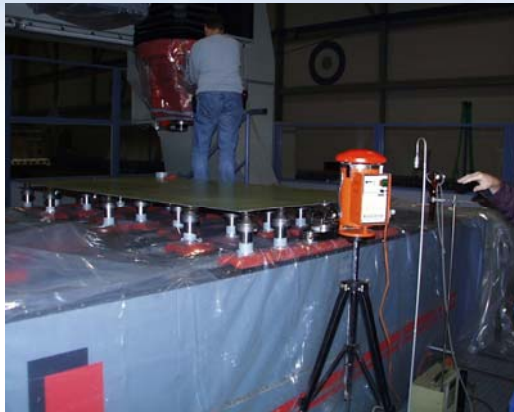
Preparation Milling station, assembling measure points for dust-emission measurement
