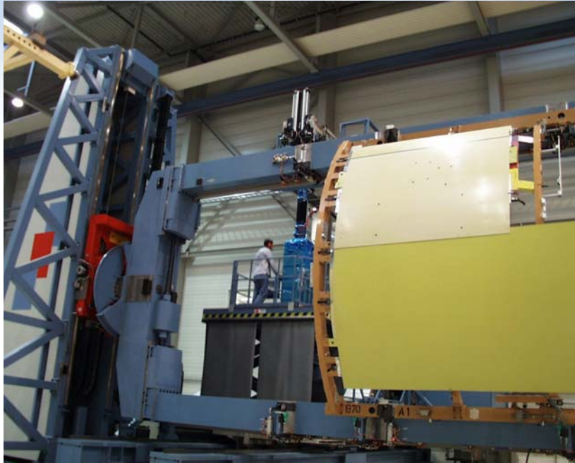
Door-frame panel on automatic riveter
