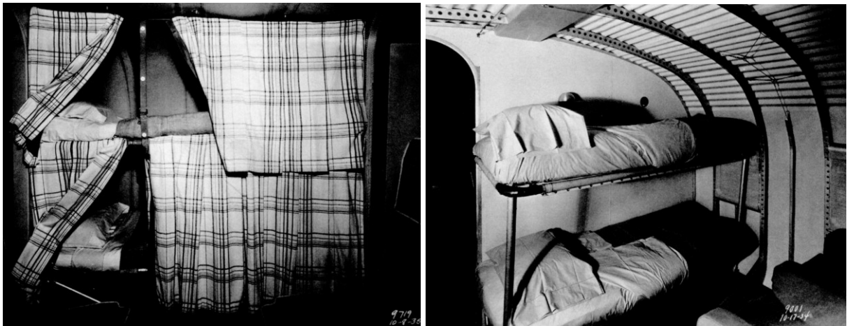
Figure 3.10 Martin M-130: Night setting with upper and lower berth beds – with and without curtains (Hühne 2016)
