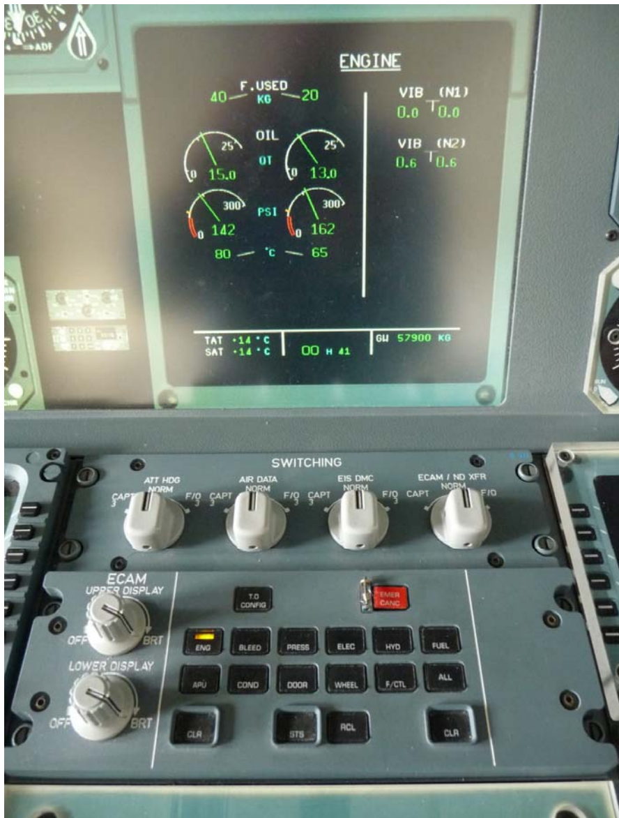
ECAM Control Panel and System Display – Here: Engine Page
